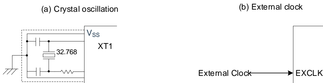
Figure4-14: Example of an external circuit for XT1 oscillation circuit
